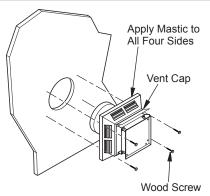
Figure 10 - Installing Horizontal Vent Cap (Noncombustible Exterior)
